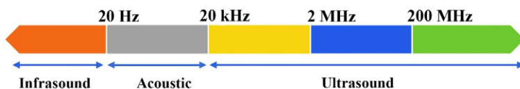
Fig. 1 Ultrasound range diagram. Adopted from S. Arefi-Oskoui, A. Khataee, M. Safarpour, Y. Orooji, V. Vatanpour, A review on the applications of ultrasonic technology in membrane bioreactors , Ultrason. Sonochem. 58 (2019) 104633, with kind permission of Elsevier.
